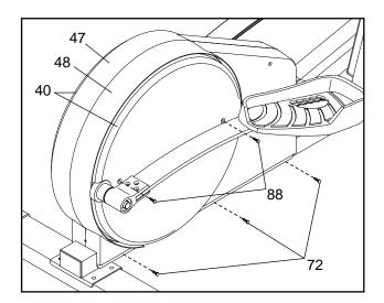
Next, locate the Reed Switch (50). Turn the Flywheel (37) until the Magnet (55) is aligned with the Reed Switch. Loosen, but do not remove, the indicated Screw (72). Slide the Reed Switch slightly closer to or away from the Magnet. Retighten the Screw. Rock the Flywheel forward and back just enough that the Magnet passes the Reed Switch repeatedly. Repeat until the console displays correct feedback. When the Reed Switch is correctly adjusted, reattach the side shields and the pedal disks.
